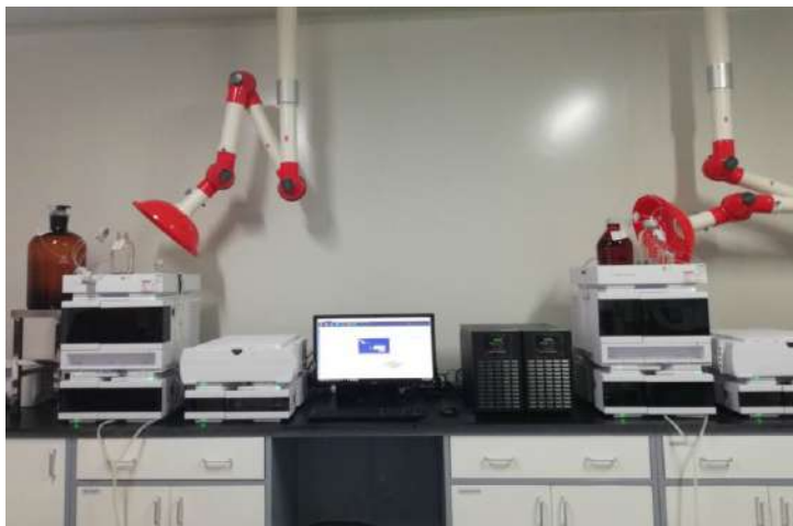
HPLC mainly used for assay and related substances testing.
